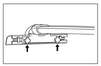
Your vehicle may be equipped with a roof rack system. To adjust the crossrails, turn both knobs on each side of the crossrail counterclockwise until it moves freely. Once the crossrail is in place, turn both knobs on each of side of the crossrail clockwise until it is secure.
